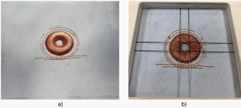
Fig. 1. Textile resonator: a) top view and b) bottom view
