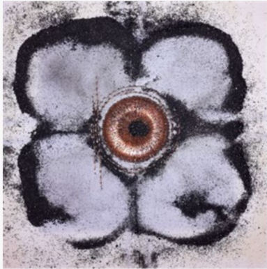
Fig. 2. Chladni sound figure on textile resonator
